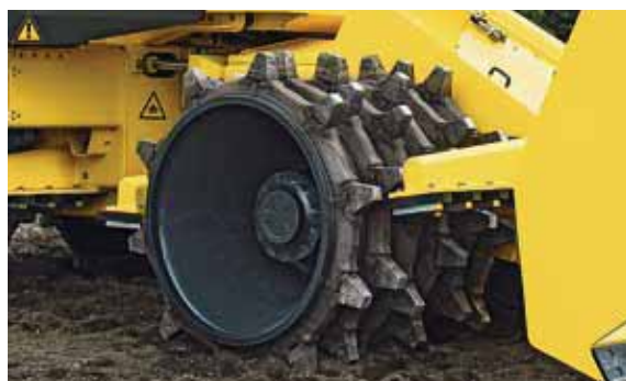
Welded wheel bodies with inner taper on both sides for optimum stability.
