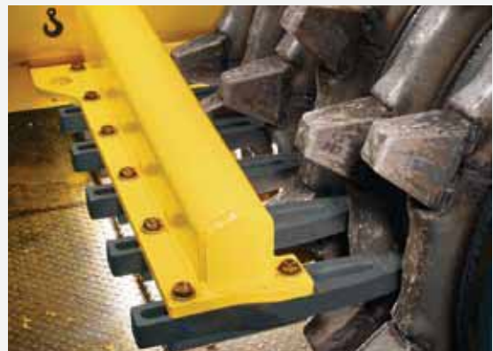
Clean wheels with effective scrapers (optimum compaction).
