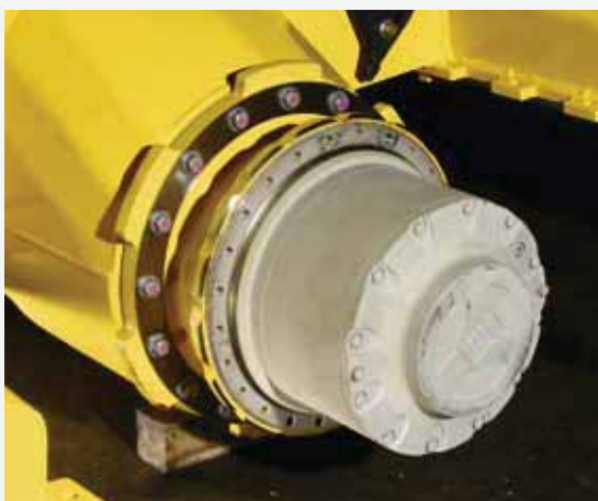
Two independent braking systems (hydrostatics used for service brake, multiple discs for the parking brake).
