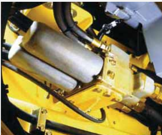
Electronic monitoring of hydraulics return filter system.
