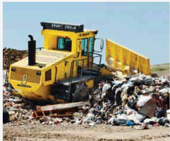
Optimum compaction with the oscillating joint, providing good load distribution to the compaction wheels.
