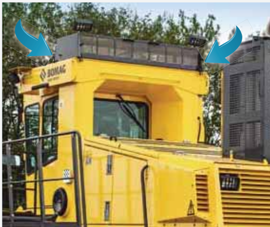
High level suction for cooling and combustion air with minimum dust levels.
