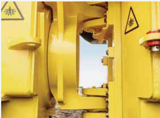
High traction with the oscillating articulated joint (continuous ground contact).
