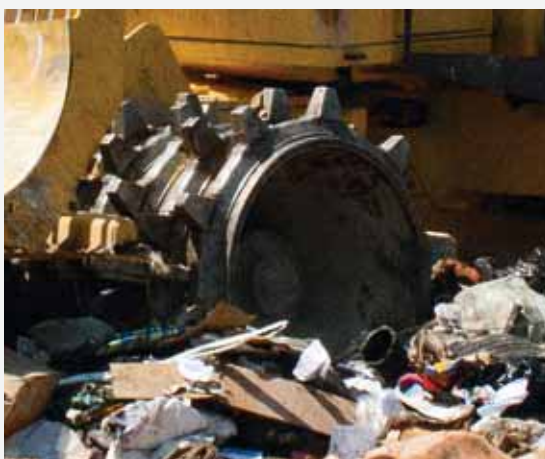
Scrapers guarantee clean wheels and high compaction.
