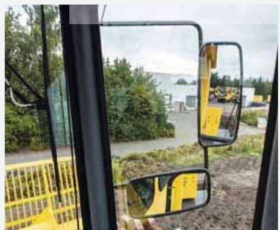
Large mirrors on both sides combined with large glass areas for excellent all-round visibility.
