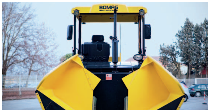
With the BOMAG SIDEVIEW system, the finisher needs just one seat and one operating console.
