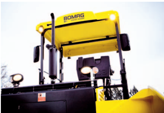
Lighting up: the finisher is fitted as standard with powerful all-round lights.
