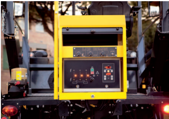
Always in view: screed release and temperature setting.
