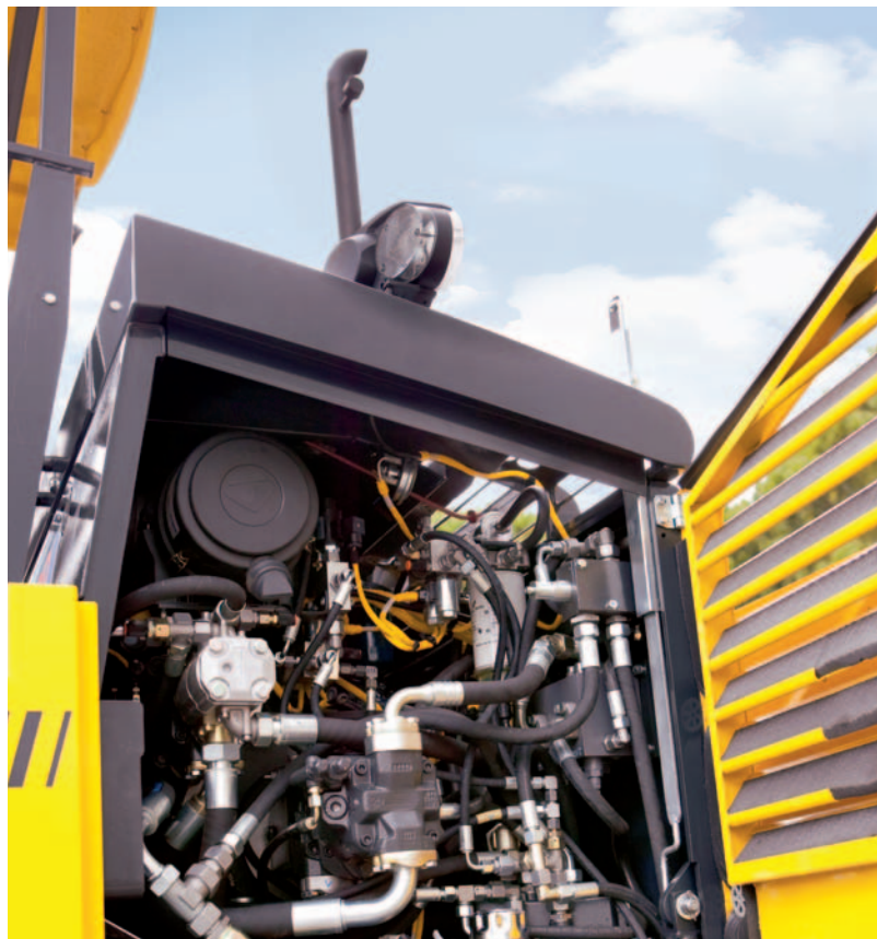
... clear access to all hydraulic and engine components.
