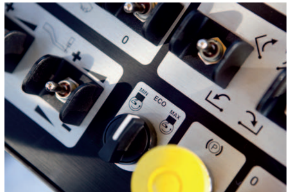
Cost-saving technology: BOMAG ECOMODE reduces fuel consumption, pollution and noise emissions.
