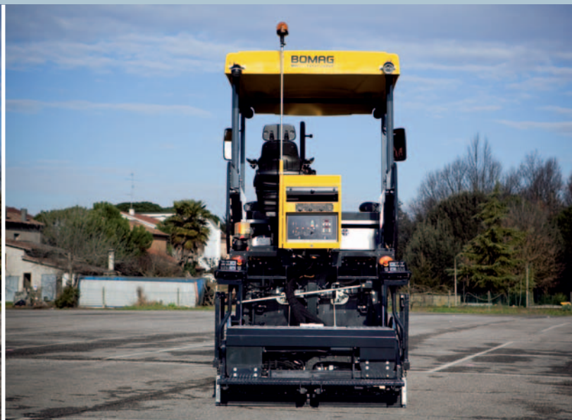
Minimum mat width with basic screed: 1.70 metres.
