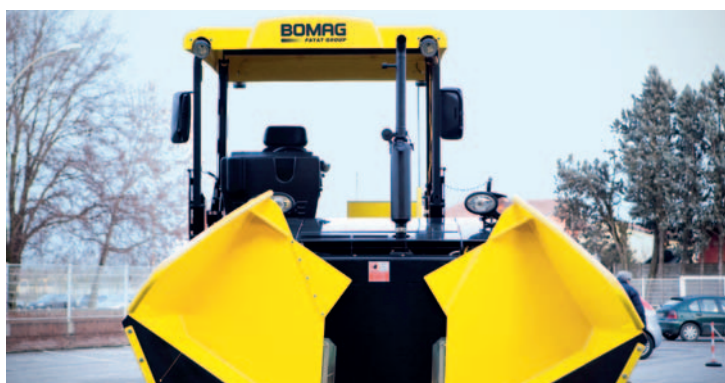
A change of perspective: the BOMAG SIDEVIEW system gives a lateral overhang of up to 40 cm.
