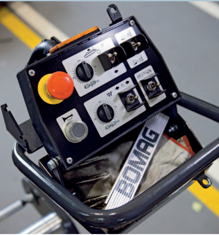
User focus: the rotating side-mounted operator's station with ample shelf space.
