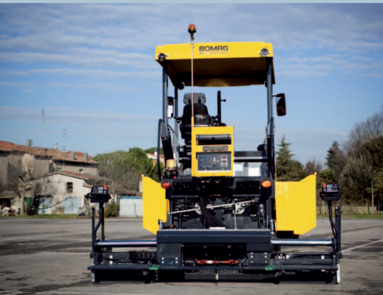
Maximum mat width with basic screed: 3.40 metres.
