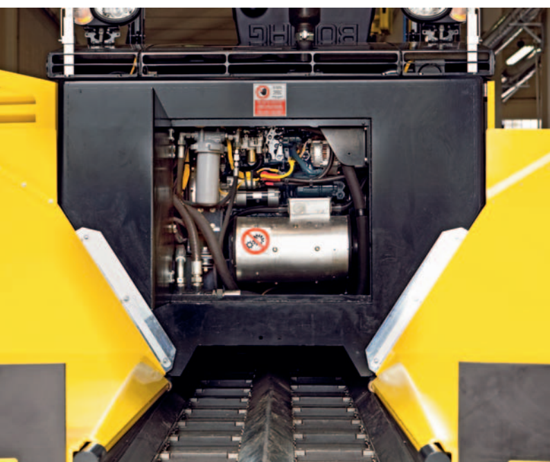
A 3-phase alternator with an output of 13 kW cuts heat-up time.
