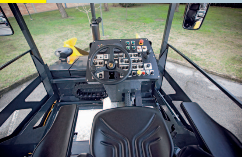
The visibility is clear: all-round vision from the operator's platform.
